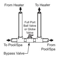
Figure 14. Auxiliary Bypass Valve.
